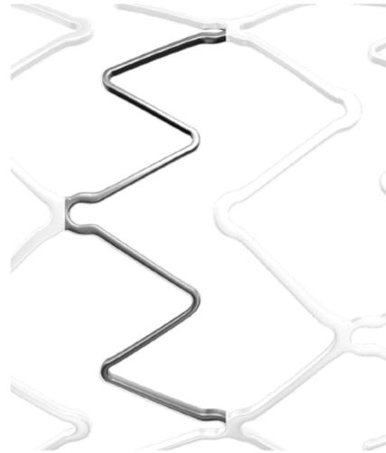
The **40µm** ultra narrow "Z" struts provide flexibility and conformability
